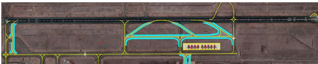
Figure 72: Phase 2 Taxiway Development Works – Extension of PTT, Link Taxiways and RETs
